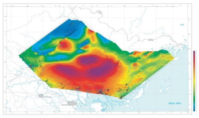
Figure 3b. Total field Magnetic Intensity Map of An Chau trough.
