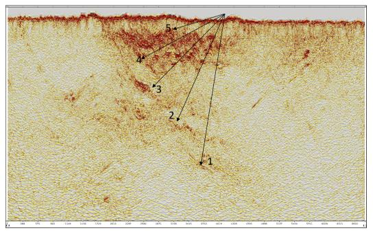
Figure 4. Define 5 main reflection surfaces on seismic data.
