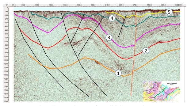
Figure 9. Paleozoic basement (horizone#3) was uplifted in center of seismic section.
