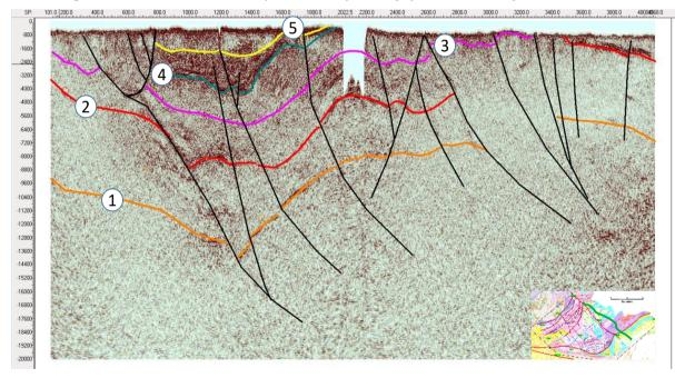
Figure 10. The seismic data shows that there is no fold in sediment located between horizon#4 and horizon#5.
