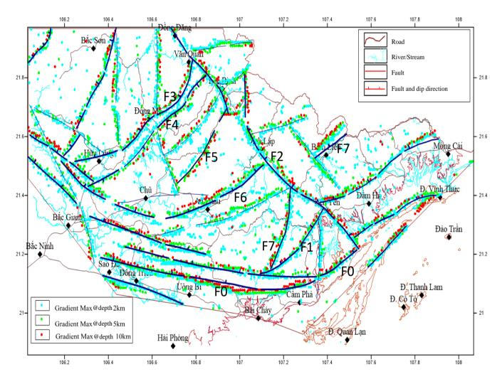
Figure 6. Defining faults systems and dip direction base on Maximum horizontal Gravity Gradient Map.
