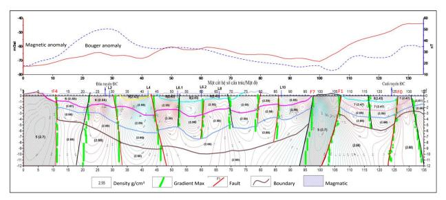
Figure 7. Defining faults and dip direction on Structure-Gravity density-Magnetic suscepcibility section.
